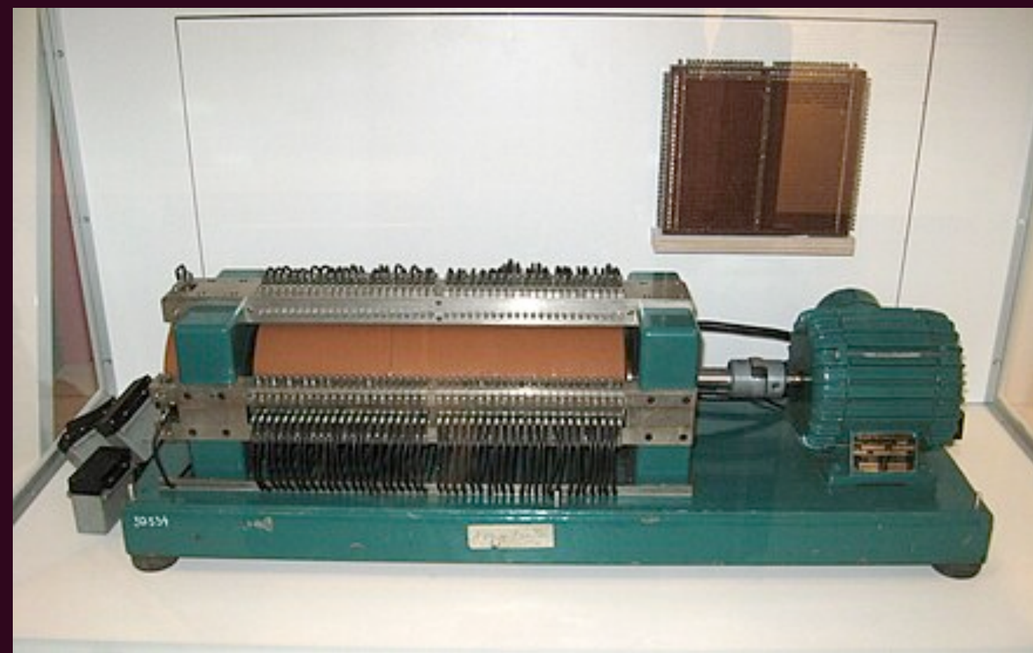
Drum memory from Sweden's first binary computer
